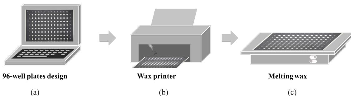
Figure 1. Schematic of the detailed procedure for making P-ELISA plates via wax printing: a) design 96-well plate pattern and layout design; b) wax printing onto filter paper (Whatman grade no. 1); c) wax melted by heating to generate hydrophobic barriers.
