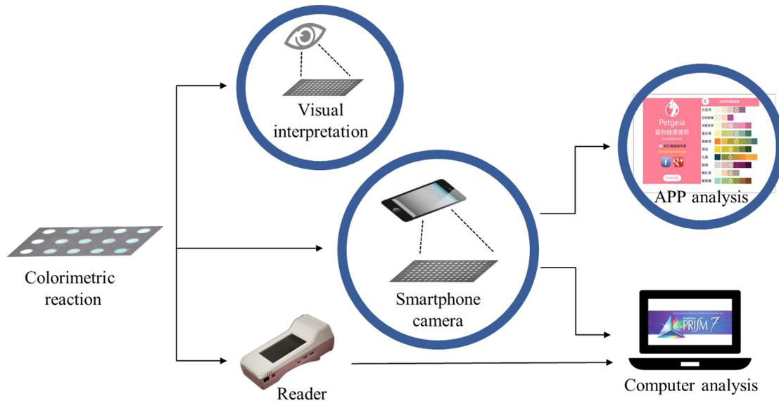
**Figure 4. Color-based signal recording methods: 1) visual interpretation; 2) specific reader; 3) smartphone camera.**
