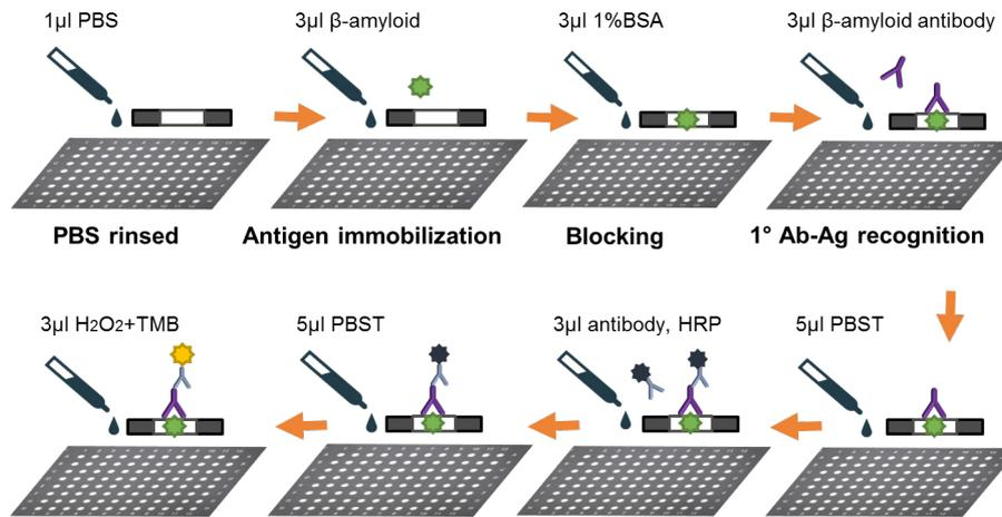
Figure 2. Schematic of the paper-based ELISA procedures for the detection of  $\beta$ -amyloid concentration.
