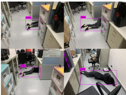
Figure 6. They were body cover 70%, body cover 50%, body cover 30% and body cover 0% of the abnormal behavior detection results
