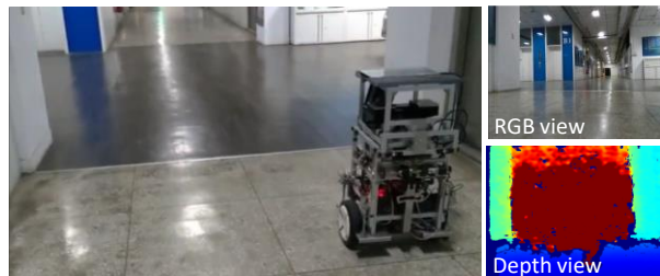
Fig. 1. The proposed auto-steering framework utilizes the front depth views to directly generate steering commands without environmental modification.
