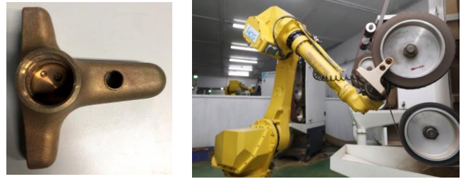
Fig.5. (a) HCG brass faucets (product type: 3720). (b) Fanuc M-710iC/50E grinding robot cell.
