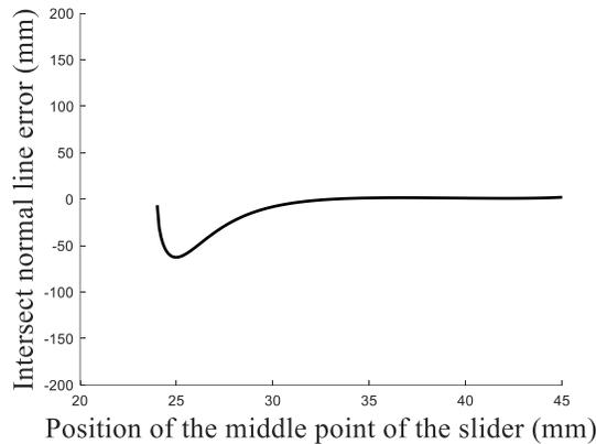
Figure 8. Variation in error of the intersect point of two normal lines of wheel links ( $K_w$ ) to the axle of the back wheel
