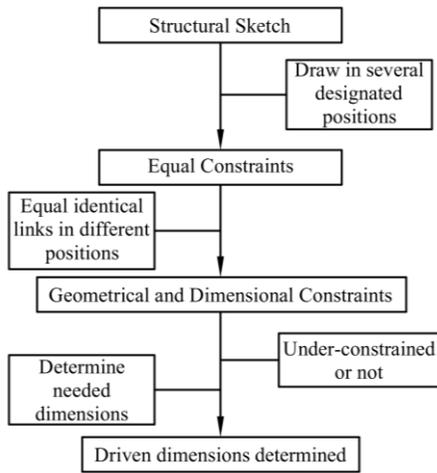
Figure 6. Geometric constraint programming
