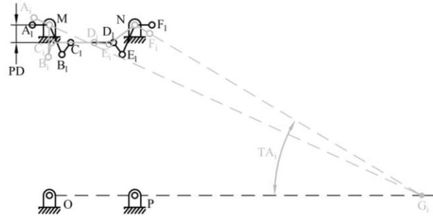
Figure 7. Six-bar linkage in its reference configuration and the  $i^{\text{th}}$  displaced configuration for Ackerman geometry
