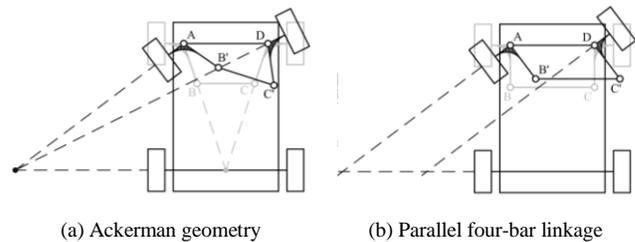
Figure 1. Steering mechanism using four-bar linkage
