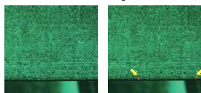
Original Images AI Detection Results Fluorescent Magnetic Particle AI Detection that Overcomes Misjudgment due to Residual Particles
