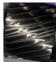
A Conventional Imaging Setup Often Leads to Reflection
