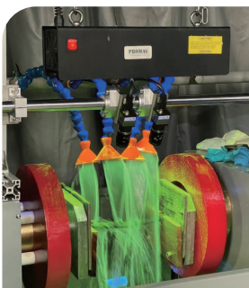
Fluorescent Magnetic Inspection Imaging Module
