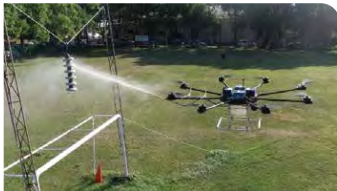
Redundant Flight Controller Applied to Insulator Cleaning
