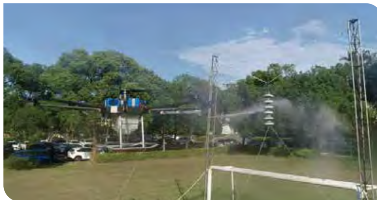
Drone-Based Insulator Cleaning Operation
